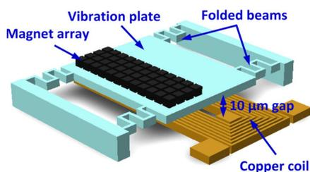
**Figure 1.** Schematic view of an electromagnetic energy harvester [1]
