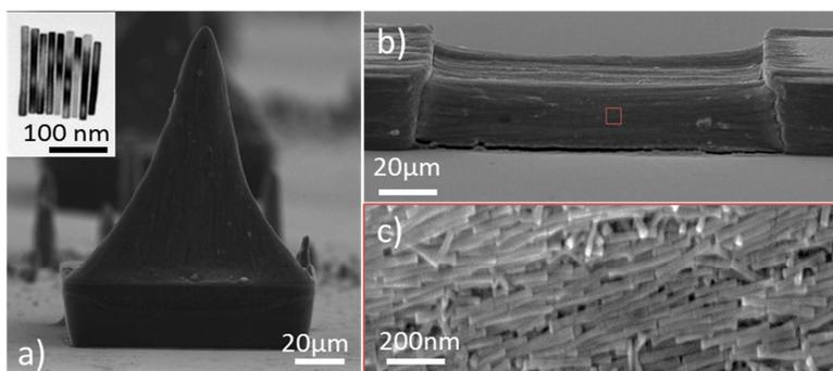
**Figure 2.** Electron microscopy images of permanent magnets with a) perpendicular and b) planar magnetization. These magnets were prepared by controlled evaporation of a suspension of Co NRs (insert figure a). c) Magnified view of the magnet revealing the alignment of the NRs.
